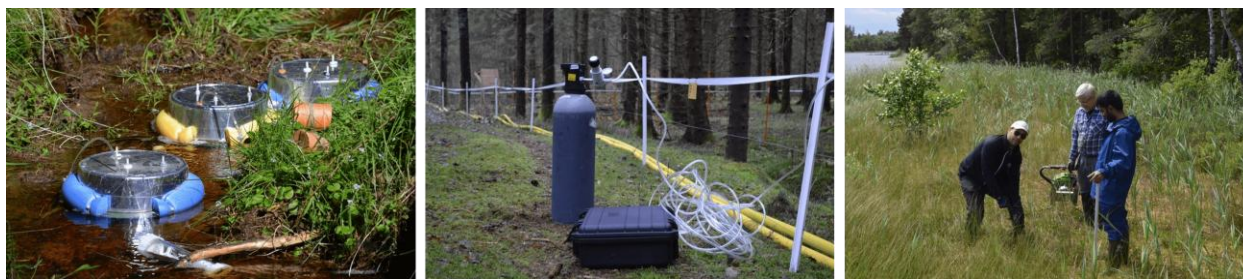
From left to right: Floating chambers to measure greenhouse gas fluxes in the streams within Skogaryd Research Catchment; Propane gas injection for gas transfer velocity measurements; Drilling the ground for installing gas equilibrators in the shore of the lake Erssjön at Skogaryd (photo credit: Sivakiruthika Balathandayuthabani)
